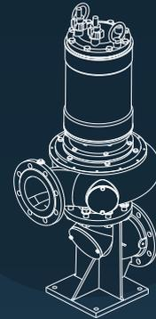
Monoblock design with standard motor (horizontal, vertical)
