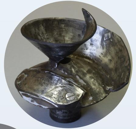
Unbalanced impeller (weldment)
